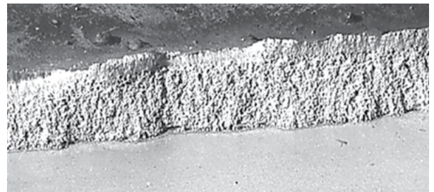
Aluminum weld with proper weld preparation shows no pores.
